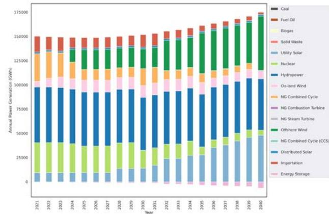
Fig 5 Annual electricity generation by source, electricity loss from energy storage units, and net electricity importation, according to the operations simulation .
