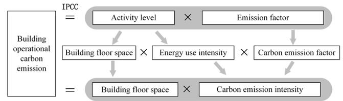
Fig 1 Building carbon emission calculation model.
