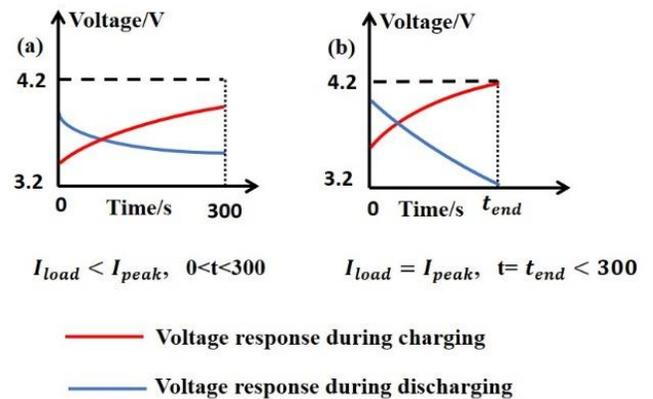
Fig. 1 The loading current and voltage response of battery during a RW step. (a) A complete RW step with 300s; (b) RW step with the cut-off voltage triggered in advance.
