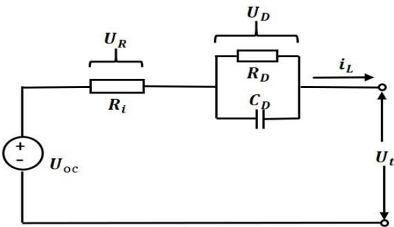
Fig.3 The 1-RC equivalent circuit model of lithium-ion battery
