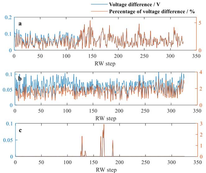
Fig.5 The average of the difference between calculated terminal voltage and measured terminal voltage. (a) Offline method; (b) Online method; (c) Optimization method
