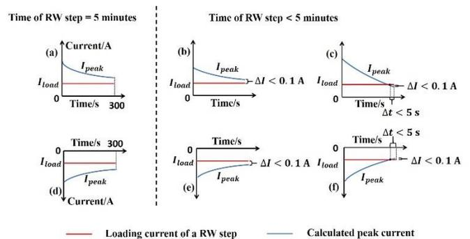
Fig. 2 The criteria for peak current calculation. (a-c) are the discharging RW steps; (d-f) are the charging RW steps.
