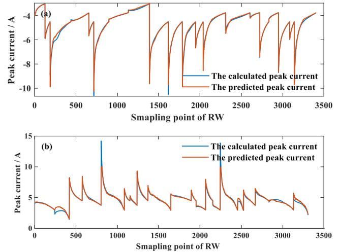
Fig. 6 The prediction result of LightGBM. (a) Charging RW steps;(b) Discharging RW steps.
