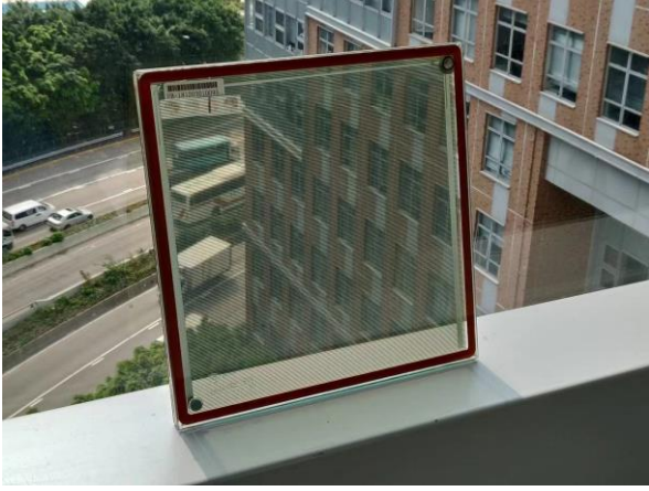
Fig. 2. The picture of the CdTe-based vacuum PV glazing
