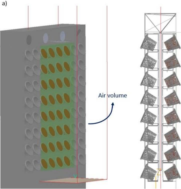
that is adjacent to the wall as shown with red-lined rectangular parallelepiped in Fig. 2a. The mesh type is cartesian for the office environment with a mesh size of 1.5 million mesh cells. The meshing structure is presented in Fig. 2b.
