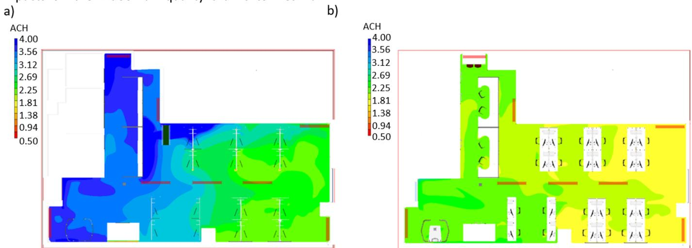
Fig. 4. ACH contours in the office environment with the green wall (1m above the floor); a) with green wall and b) no green wall.
