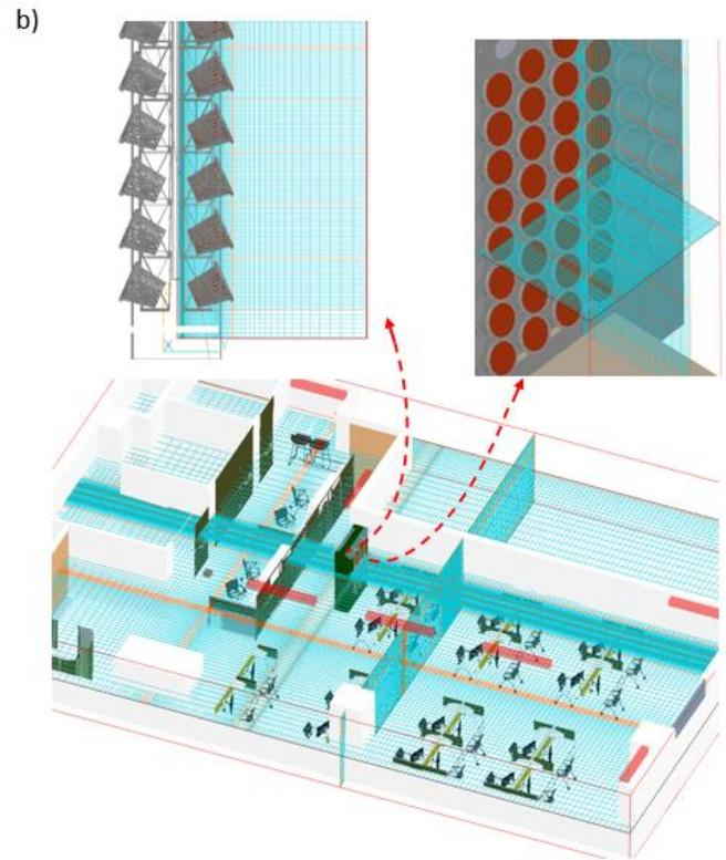
Fig. 2. The numerical model of the green wall and office environment; a) computational model and b) mesh structure.
