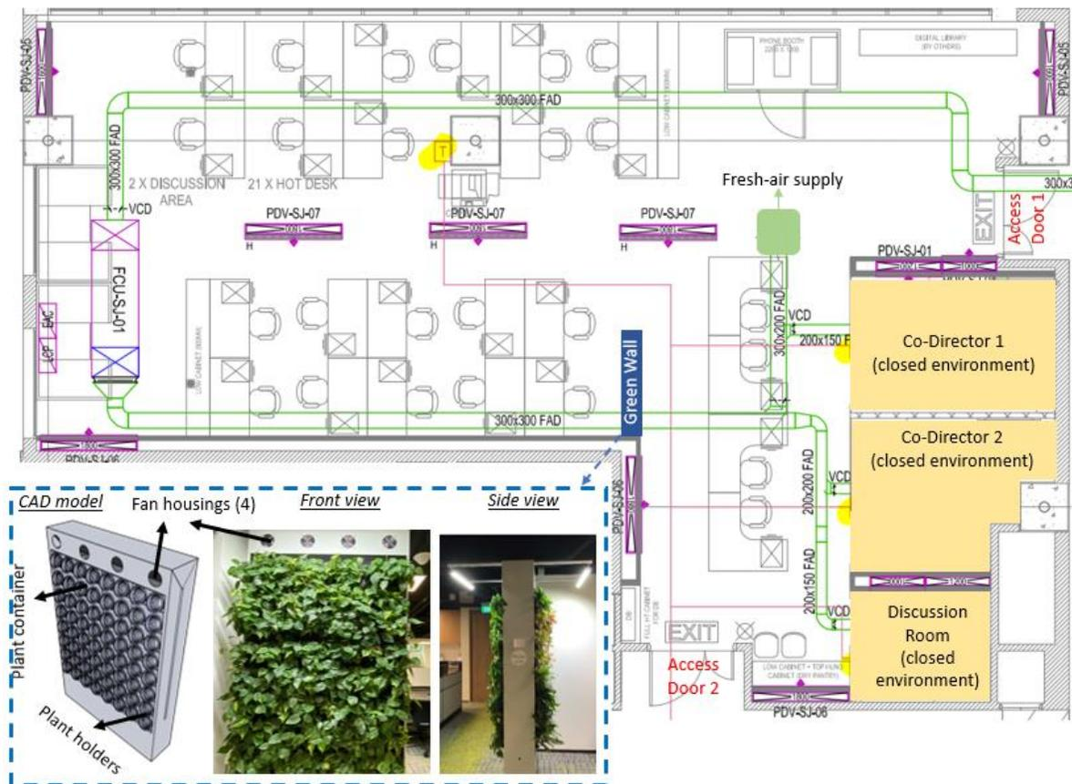
Fig. 1. The office layout and the green wall structure.
