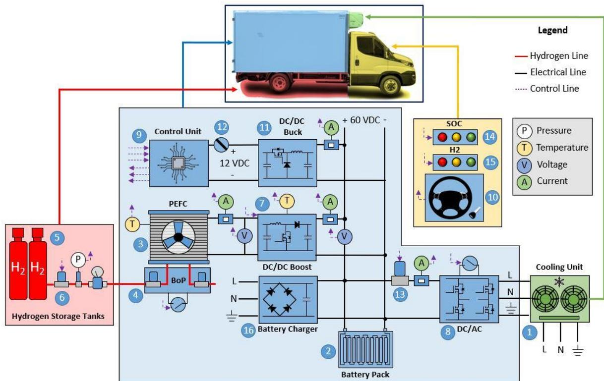
Fig. 1. Hydrogen-based APU for refrigerated van. Component layout
