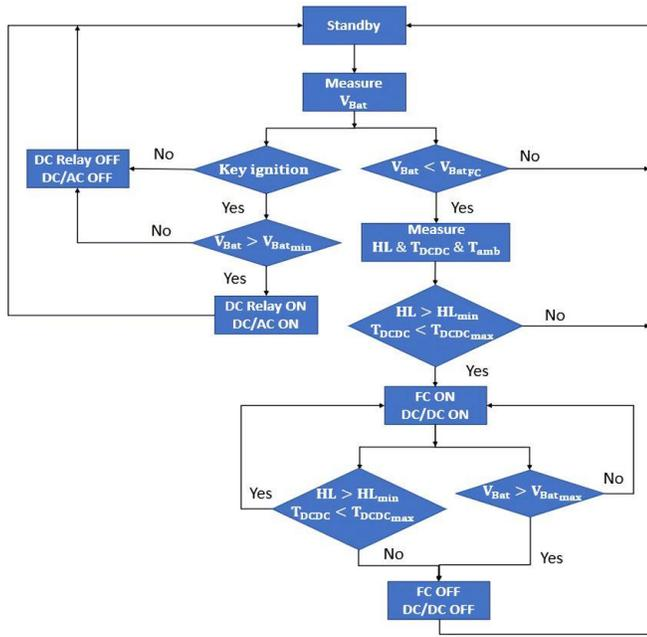
Fig. 2. EMS strategy of the developed Hydrogen-based APU.
