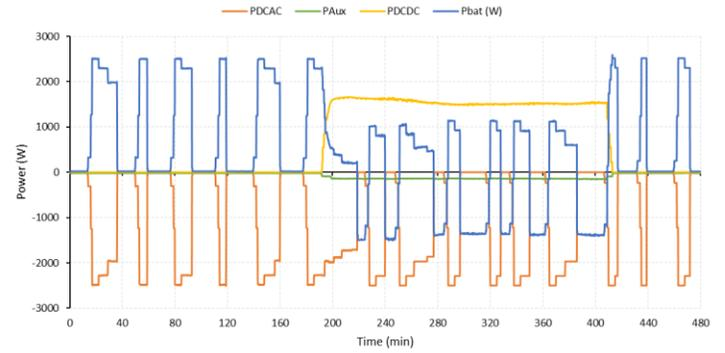
Fig. 5 Battery ( $P_{Bat}$ ), DC/AC input power ( $P_{DC/AC}$ ), DC/DC output power ( $P_{DC/DC}$ ) and auxiliary consumption ( $PAux$ ) power profile.
