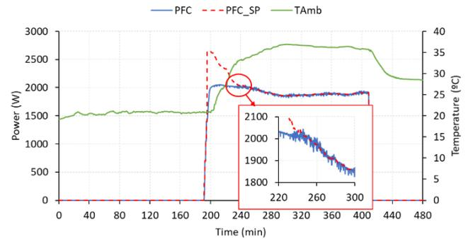
Fig. 7. PEFC generation (PFC), PEFC power setpoint (PFC\_SP) and ambient temperature (TAmb) profile.
