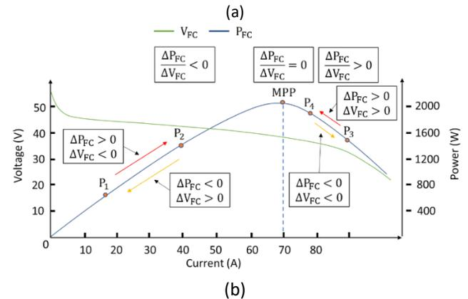
Fig. 3. PEFC control law (P&O algorithm); (a) flowchart; (b) P&O principle
