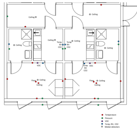
Fig. 3. Layout of the sensor network in two of the four apartments in Testbed KTH, layout 1.0 (2018-2020). The deployed sensor network allows detailed monitoring of the Indoor Environmental Quality (thermal comfort and air quality) in parallel with the mapping of the resource flows.
