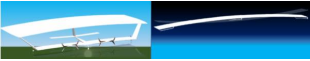
Fig. 3: The Flying Leaflet (FLT) and the Flying Leaf (FL) formed from 11 FLT's with 8 carriers released.
