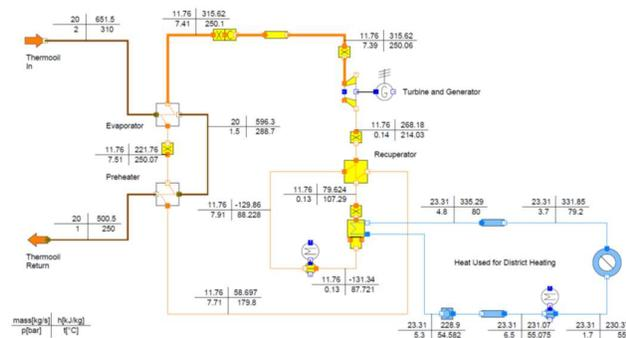
Figure 2. Schematic diagram of the model for the ORC of the B CHP plant
