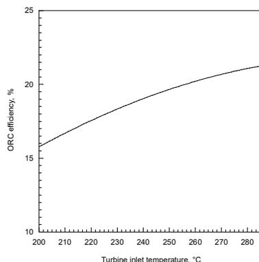
Figure 3. Modeling results of the ORC efficiency as a function of turbine inlet temperature.
