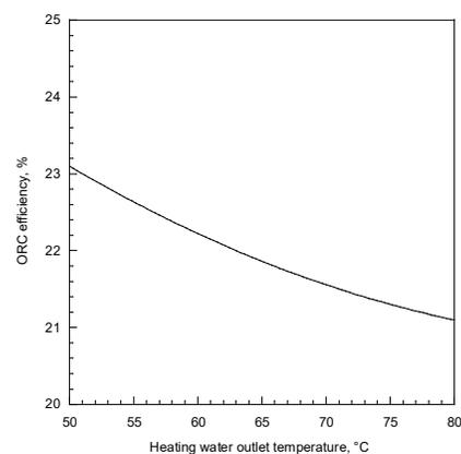
Figure 4. Modeling results of the ORC efficiencies as a function of heating water outlet temperature.
