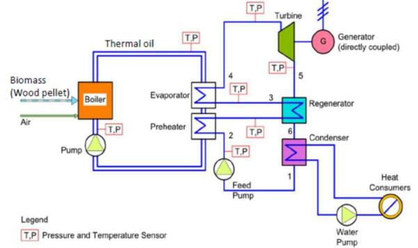
Figure 1. Schematic diagram of a BCHP system using ORC
