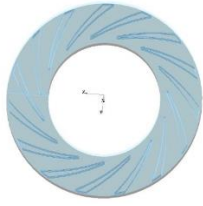
Fig. 4. The first stage has a vane diffuser
