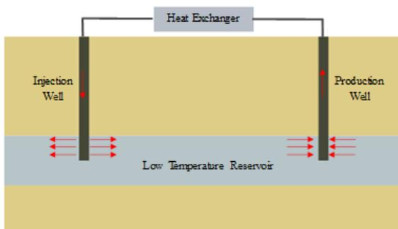
Figure 1. Conceptual schematic of an AGES system
