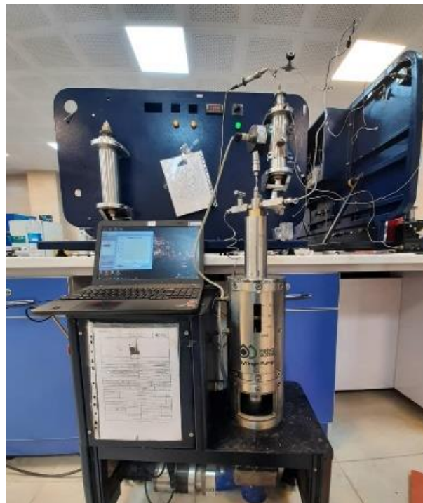
Figure 1: A view of the set-up used for injection of SC- CO_2 into selected limestone core samples.
