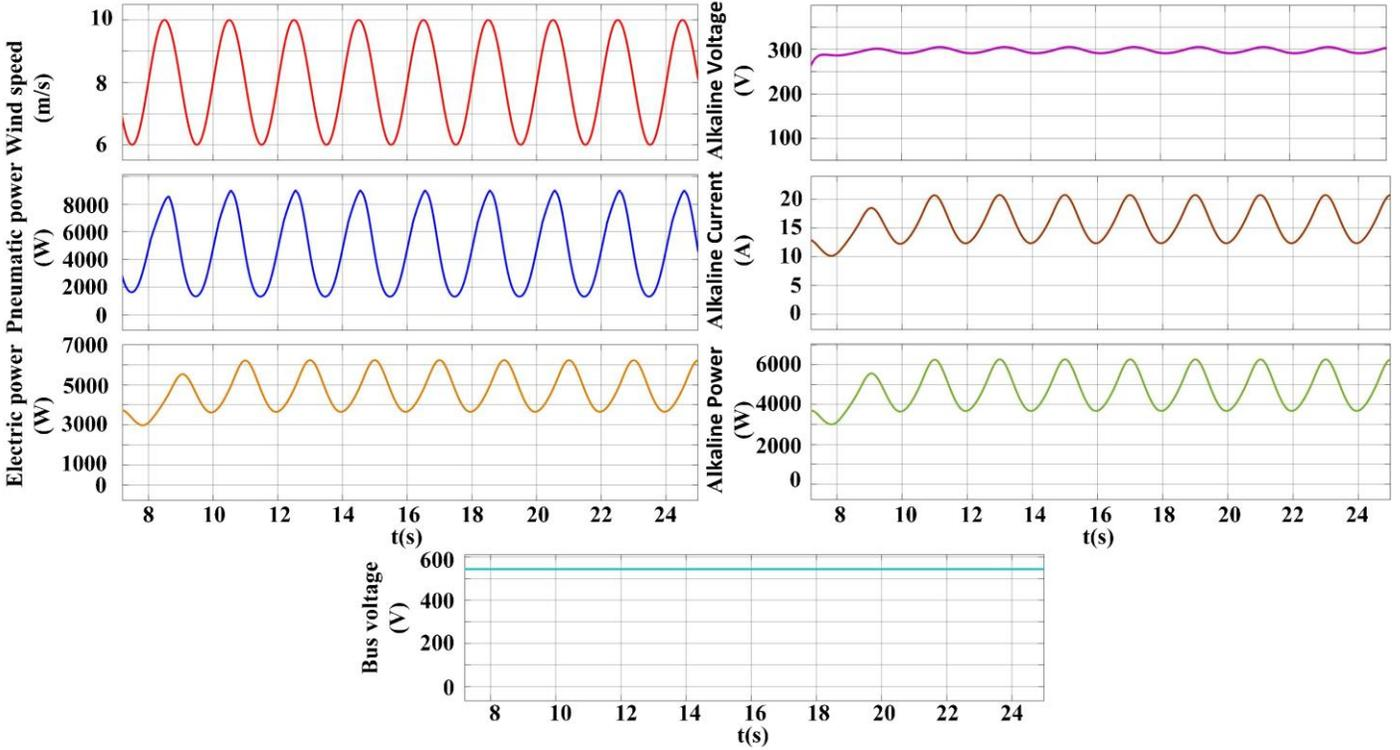
Fig. 2 System simulation results under sinusoidal wind input
