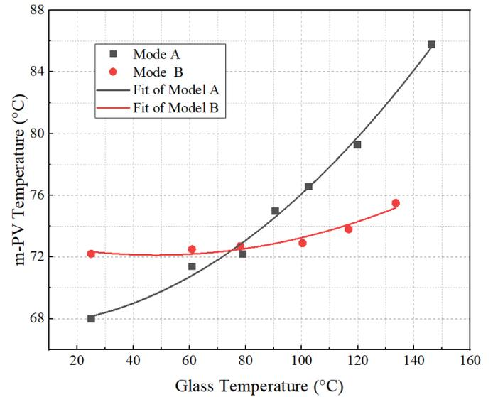
Fig. 4 Comparisons of temperatures of m-PV panels with and without high-reflective coating
