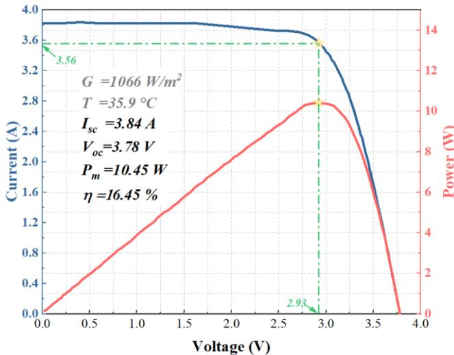
Fig. 3 I-V curve of PV panel
