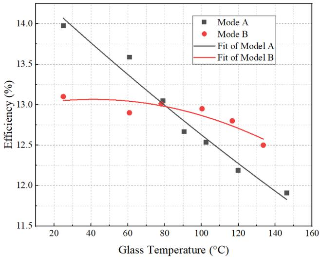
Fig. 5 Comparisons of photoelectric efficiencies of m-PV panels with and without high-reflective coating
