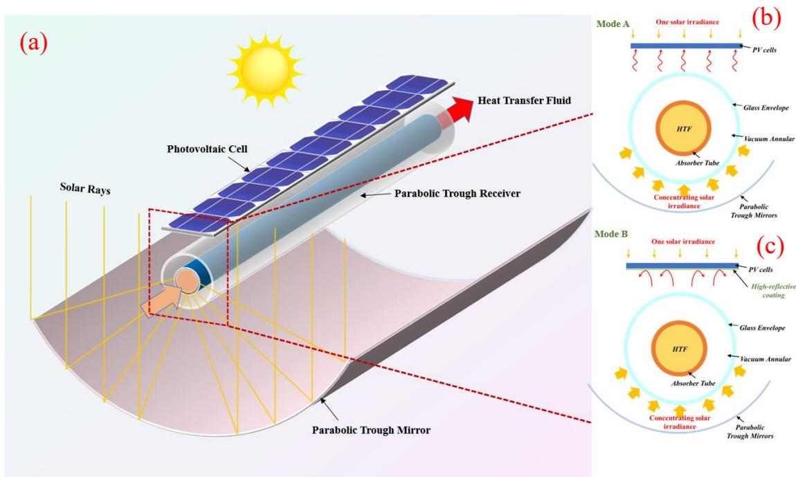
Fig. 1 (a) Schematic diagram of hybrid PTC-PV system and two modes of PV panels: (b) PV panels without high-reflective coating and (c) PV panels with high-reflective coating
