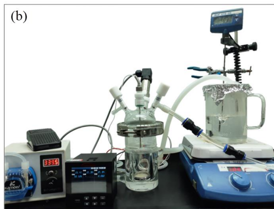
Fig. 2. (a) The schematic of the experimental setup for the measurement of CO_2 uptake of MECS in a constant-volume vessel. PT and TT are the pressure and temperature transmitters connected to a data logger, respectively, and TC is the temperature controller for water bath. (b) The photo of the experimental setup
