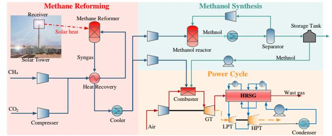
Fig. 1 Layout of the solar polygeneration system
