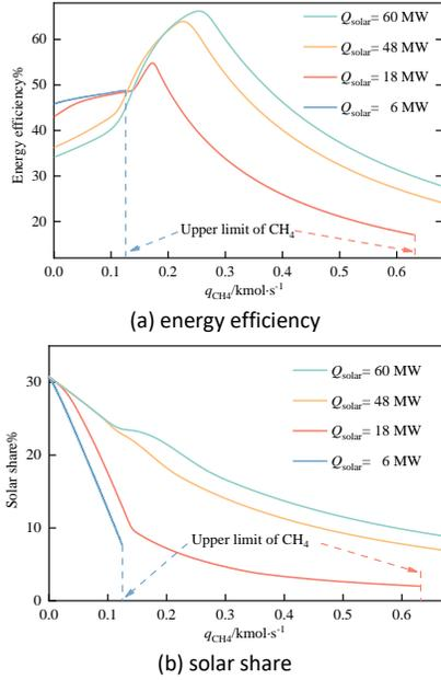
Fig.5 Effect of methane flow on energy characteristics
