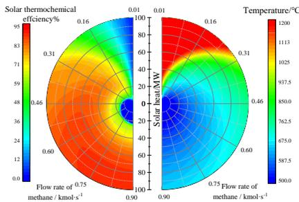
Fig. 3 Effect of methane flow and solar heat on reaction characteristics of solar MDR
