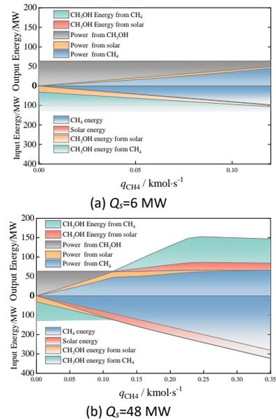
Fig. 4 Effect of methane flow on energy output
