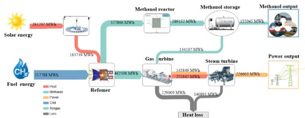
Fig. 9 The annual energy stream diagram of the system
