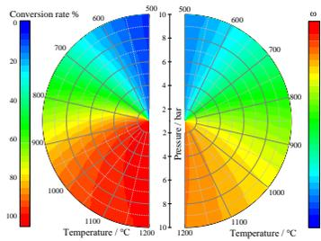
Fig. 2 Effect of temperature and pressure on reaction characteristics of MDR
