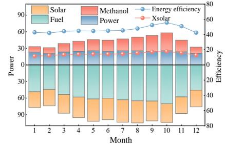
Fig. 8 The monthly energy output of the system
