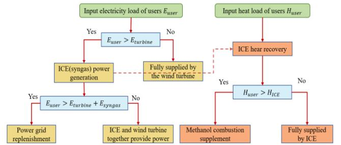
Fig. 4. The calculation flow diagram
