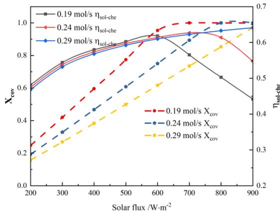
Fig. 6. Effect of DNI and methanol feed on methanol conversion rate and solar thermochemical efficiency
