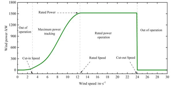
Fig. 3. Power curve of the wind turbine
