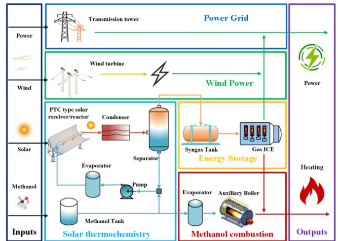
Fig. 1. Structure and workflow of the new system
