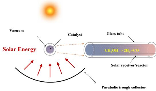
Fig. 2. Schematic of the solar receiver/reactor
