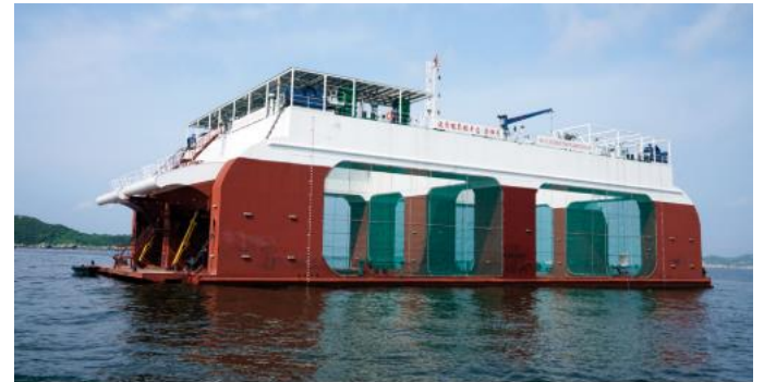
Fig. 2 Penghu semi-submersible wave powered aquaculture platform (image courtesy of Guangzhou
