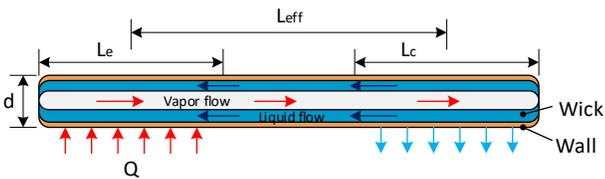
Fig. 1 Heat pipe structure
