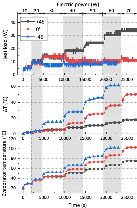
Fig. 4 Heat pipe performance at 6m/s of air velocity
