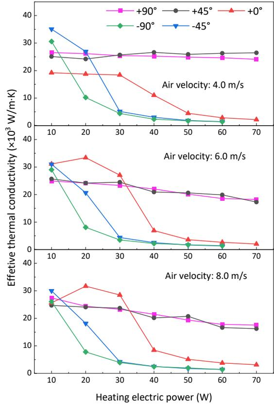
Fig. 5 Variation of  $K_{eff}$  at different conditions
