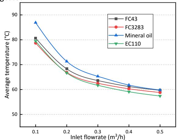
Fig.5 Effect of inlet flowrate on average temperature
