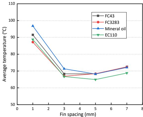
Fig.6 Effect of different fin spacing on average temperature
