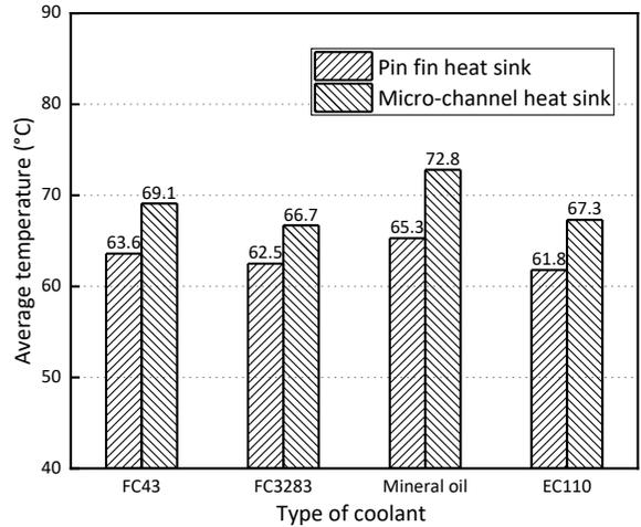
Fig.4 Effect of heat sink and coolant on average temperature
