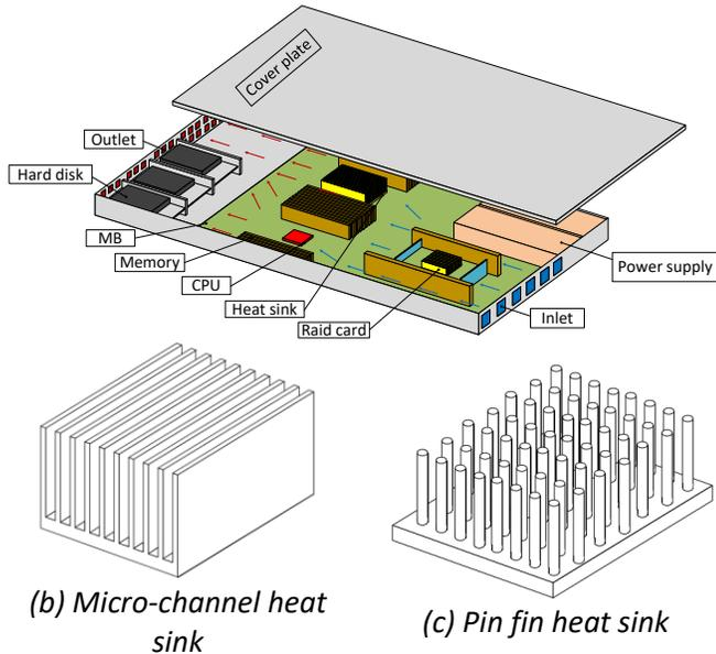
Fig.1 Models of server and heat sink
