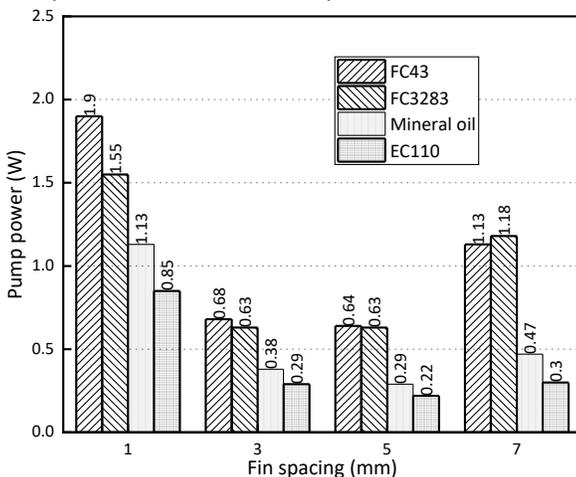
Fig.7 Pump power under different fin spacing and coolants
