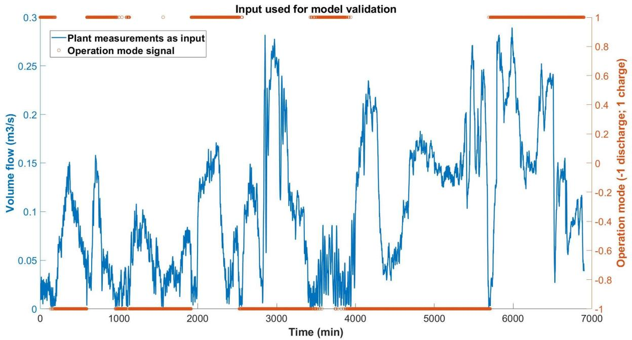
Figure 2 - Inputs used for validation - operation mode and volume flow used
