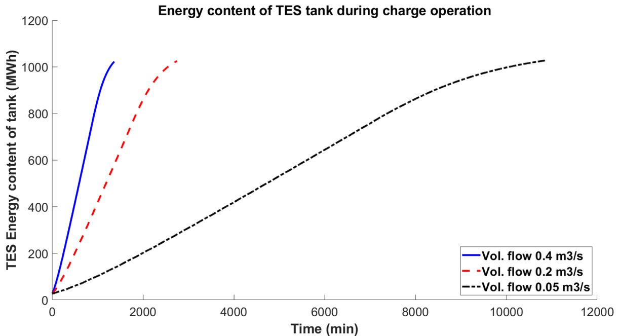
Figure 5 – Discharge operation for the analyzed tank with 3 different volume flows
