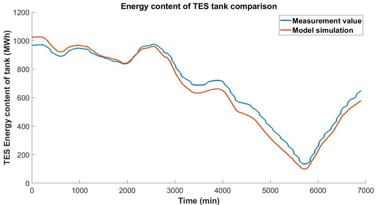
Figure 3 – Validation results for the energy content of the analyzed tank
