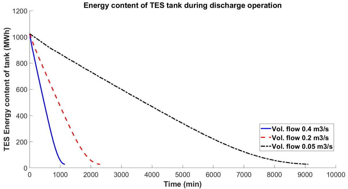
Figure 4 – Discharge operation for the analyzed tank with 3 different volume flows
