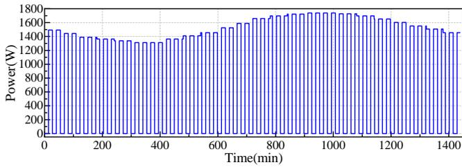
Fig. 7 Compressor power (1C)
