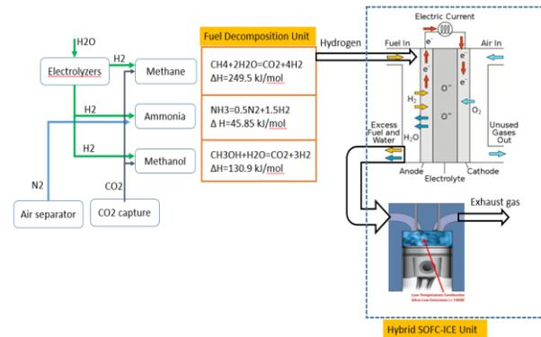
Fig. 1 low-carbon fuels applied for hybrid SOFC-ICE System diagram
