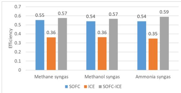
Fig. 3 Power efficiency of prime movers fueled with syngas
