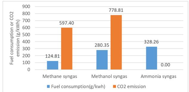
Fig. 5 fuel consumption and carbon dioxide emission
