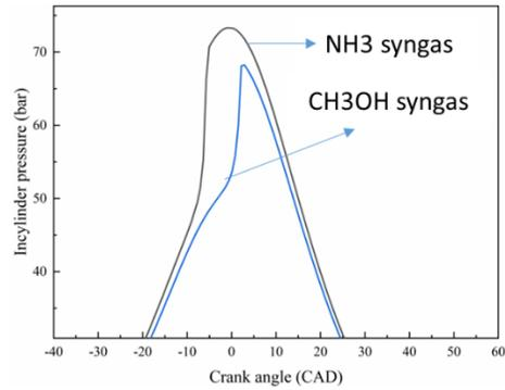
Fig. 4 in-cylinder pressure of NH<sub>3</sub> and CH<sub>3</sub>OH anode off-gas
