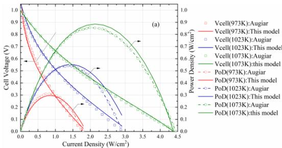
Fig. 2 The V-J curve verification
