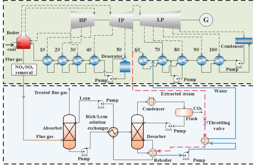
Fig. 1. Flow diagram of a 1000MW coal-fired thermal power system equipped with post combustion CO<sub>2</sub> capture
