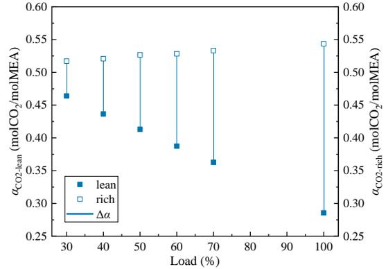
Fig. 5. Variation of lean-rich liquid loading under different power loads
