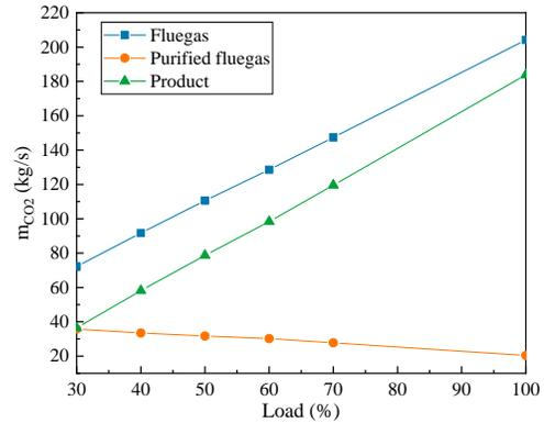
Fig. 6. Variation of  $CO_2$  mass flow rate under different loads
