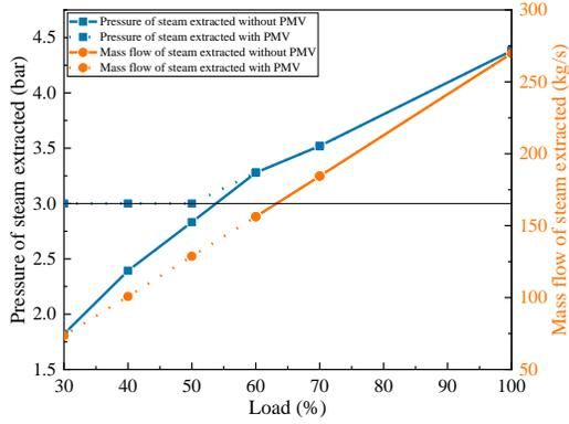
Fig. 3. Impact of steam extraction on power generation system under different loads
