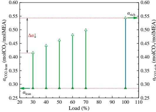
Fig. 8. Influence of flue gas mass flow on  $\Delta\alpha$
