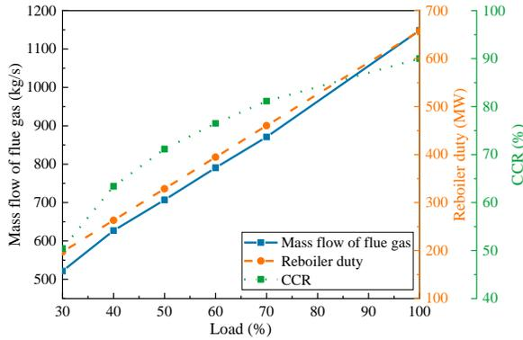
Fig. 4. The influence of changes in flue gas mass flow rate on CCR under different loads
