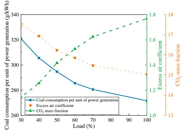
Fig. 2. Coal consumption per unit of power generation, excess air coefficient, and CO<sub>2</sub> mass fraction under different loads
