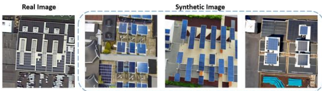
Fig. 4. The leftmost one is the real image provided as image prompt and the others are synthetic images. Synthetic Images are generated with “an overhead aerial image of photovoltaics panels mounted on rooftops” as text prompt via text-guided image-to-image generation.
