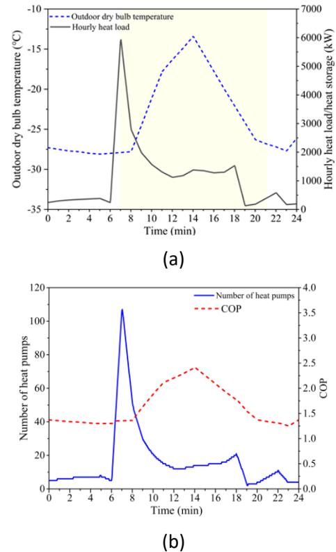
Fig. 2 (a) Hourly variations in outdoor dry bulb temperature and heat load; (b) Hourly variations in the number of heat pump and COP.
