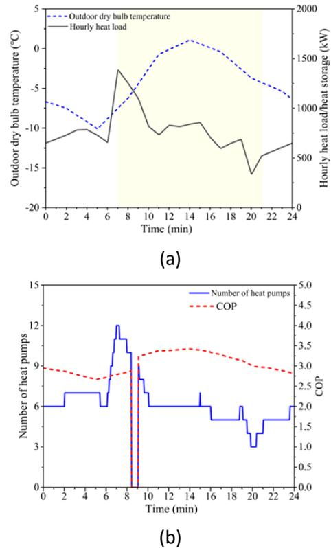
Fig. 6 (a) Hourly variations in outdoor dry bulb temperature and heat load; (b) Hourly variations in the number of heat pump and COP.
