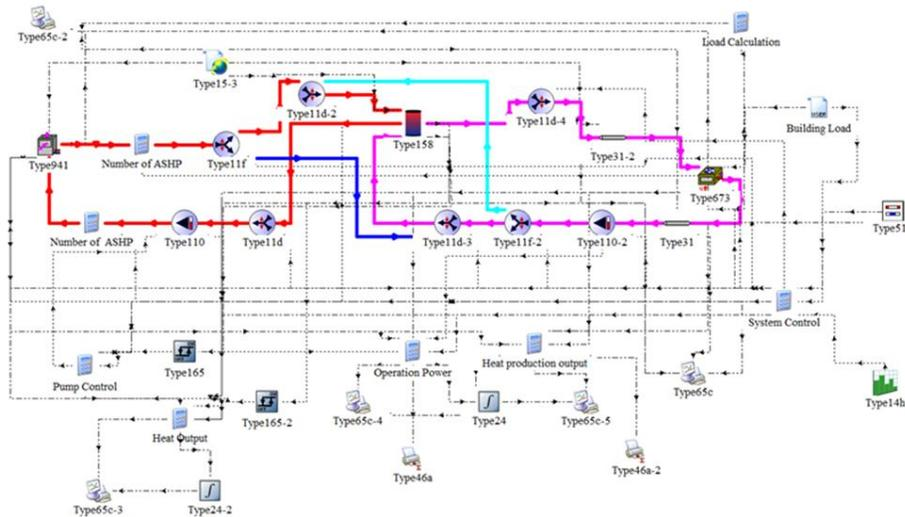
Fig. 1 The air source heat pump heating system.
