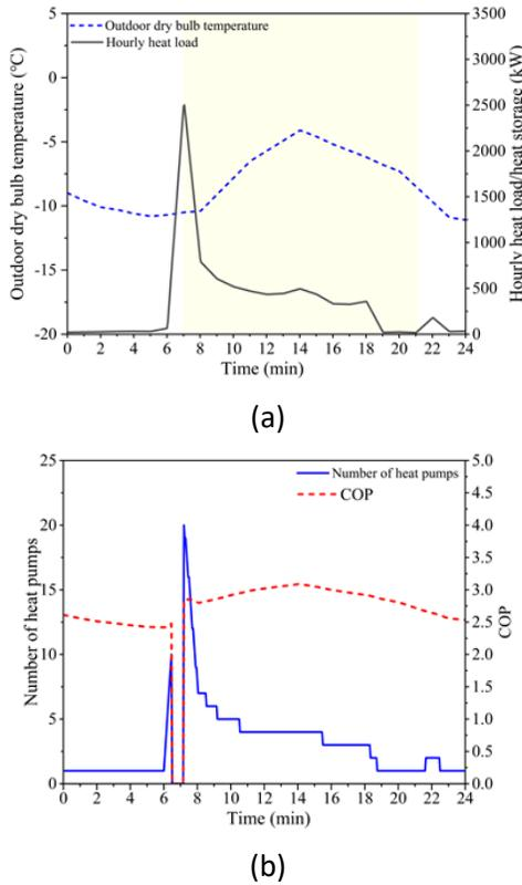
Fig. 5 (a) Hourly variations in outdoor dry bulb temperature and heat load; (b) Hourly variations in the number of heat pump and COP.
