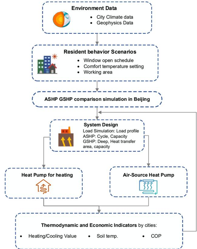
Fig. 1 Comparison framework of GSHP and ASHP
