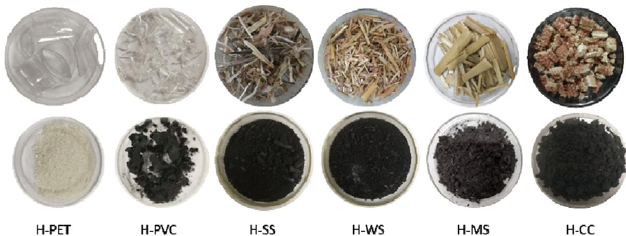
Fig 1 Image of raw samples and hydrochars
