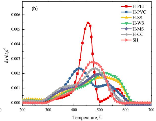
Fig 3 The combustion curves of different samples (a) Conversion rate, (b) Reaction rate
