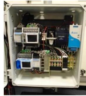
Fig 1 Grid Data Unit including  $\mu$ PMU.
