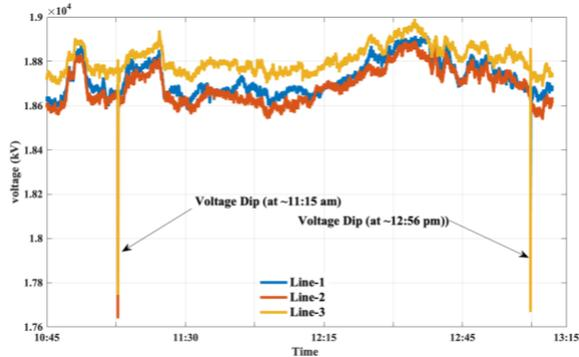
Fig. 5 Voltage dips of the  $\mu$ PMU data on the tested day.
