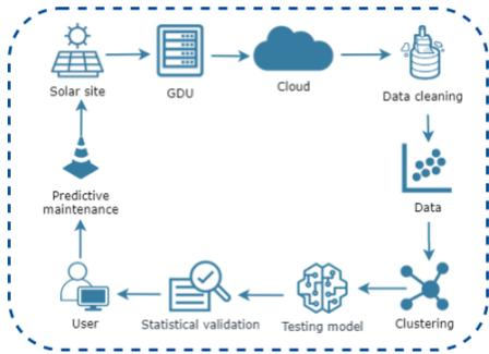
Fig. 3 Proposed flow diagram for  $\mu$ PMU data-driven based anomaly event detection.
