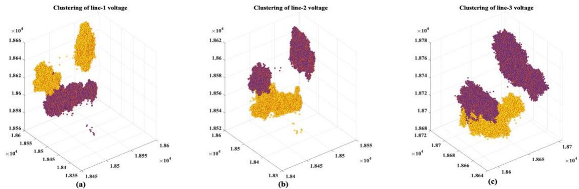
Fig 4 Clustering outcomes for three-phases voltage of a single day micro-PMU data.
