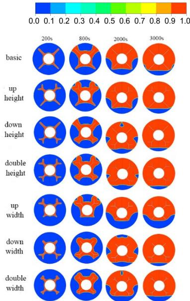
**Fig.6.** Liquid fraction distraction with the time.
