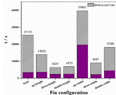
Fig.5. Total melting time and bottom melting time.
