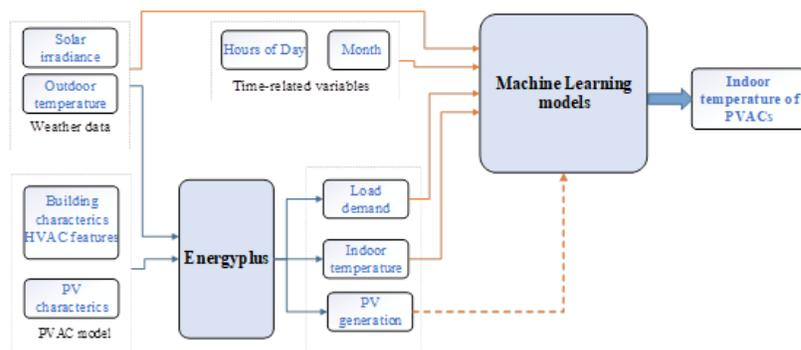
Fig. 2. A calculation framework for the indoor temperature of the PVAC system
