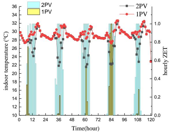
Fig. 7. Comparison of hourly ZET and indoor temperatures for PVACs in a week of July
