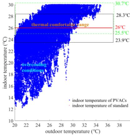
Fig. 4. The fixed and flexible indoor temperatures of PVACs in summer
