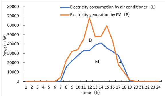
Fig. 3. Hourly energy matching of the PVAC system in Shanghai on June 1st
