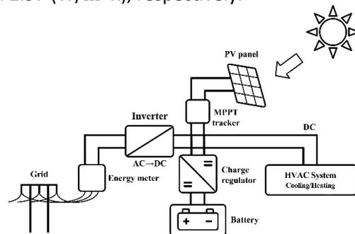
Fig. 1. PVAC system schematic
