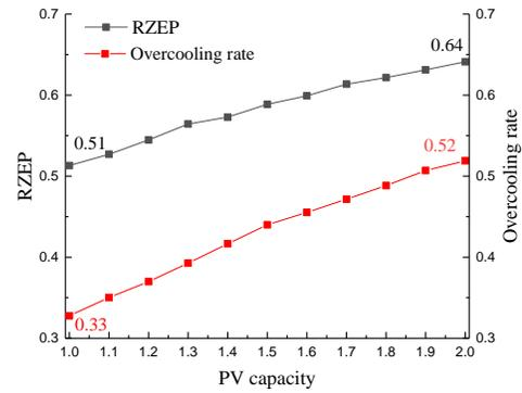
Fig. 6. RZER and overcooling rate for different PV sizes
