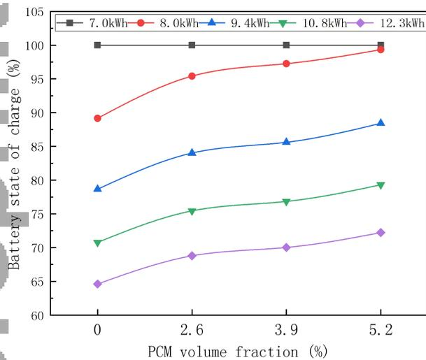
Fig 9 Hourly peak of battery SOC.
