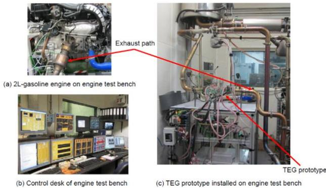
Fig 3: Experimental test setup on the engine test bench.
