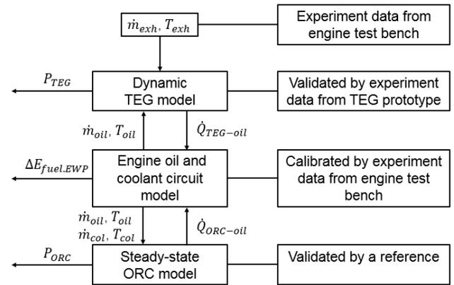
Fig 2: The model structure and variables for the semi-empirical model.
