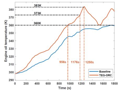
(b) Comparison of warm up characteristics of engine oil for baseline scenario and TEG-ORC system.
