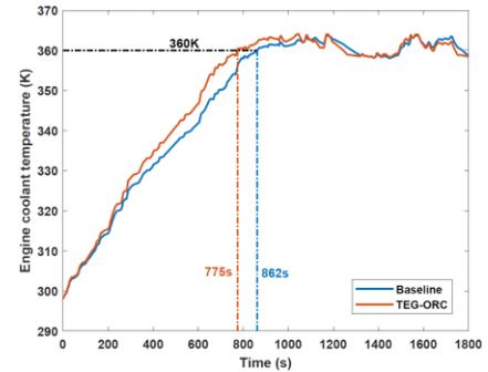
(a) Comparison of warm up characteristics of engine coolant for baseline scenario and TEG-ORC system.
