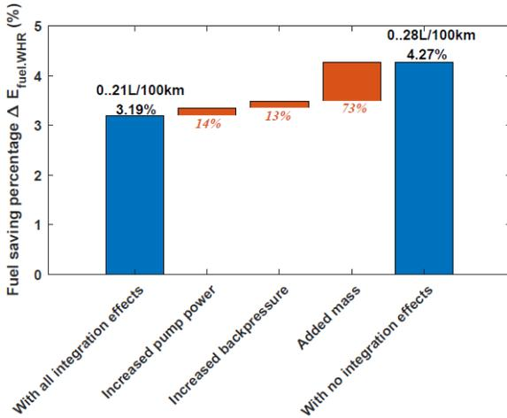
Fig: 7 Fuel saving potential of TEG-ORC system in the WLTP with and without integration effects.
