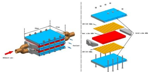
Fig A1: Structure and parameters of the TEG system [3-4].
