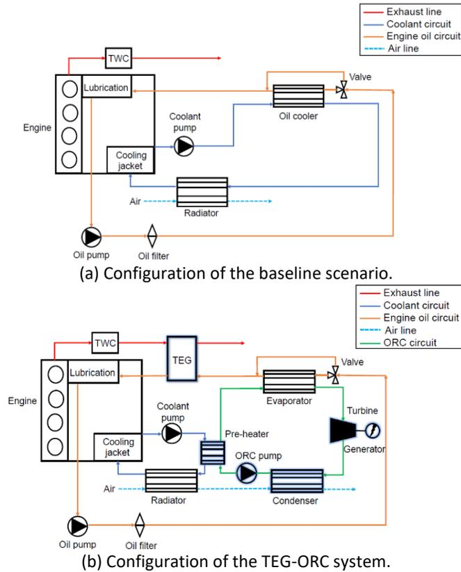
Fig 1: Comparison of layouts between the baseline scenario and TEG-ORC system.
