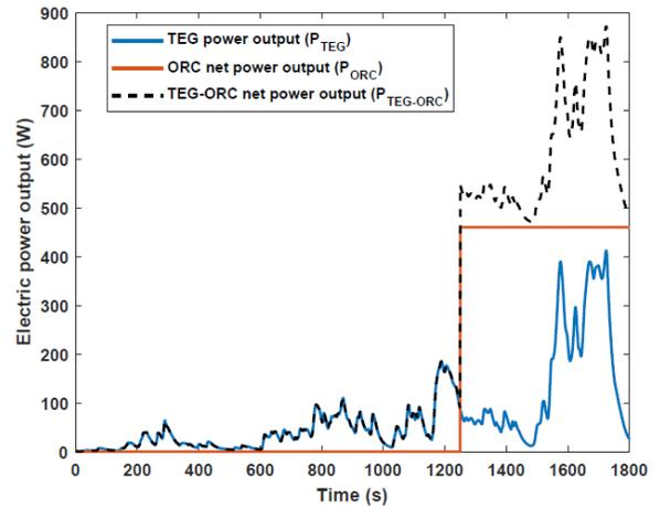
Fig 6: Electric power output of the TEG-ORC in the WLTP.
