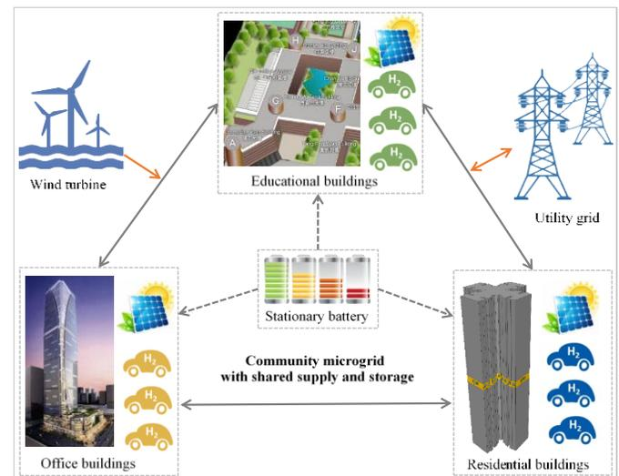
Fig. 1 Schematic of the zero-energy building community with hybrid renewable energy and storage systems
