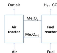
Figure 1 Schematic diagram of the chemical looping gasification process
