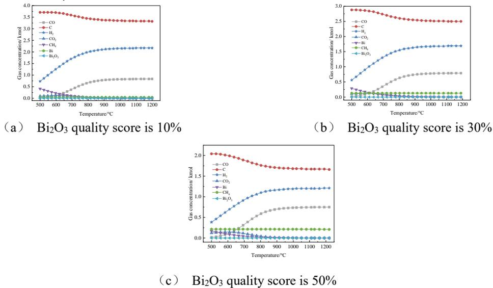
Fig. 2 Effect of temperature BC/ $Bi_2O_3$  chemical looping gasification process at different mass fractions of  $Bi_2O_3$
