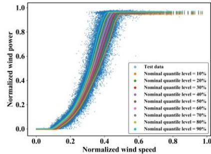
Fig 1 Results of the quantile based wind turbine power curves.
