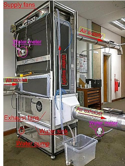
Fig. 1 Experimental rig for dew point evaporative cooler
