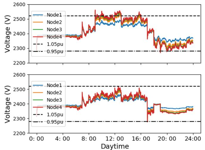
Fig 8 Voltage levels of the four-node system – (upper) before schedule-based active TES control and (lower) after schedule-based active TES control;
