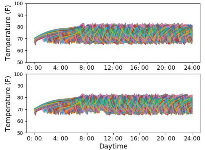
Fig 7 Indoor temperature profiles of 360 residential houses – (upper) before priority-based control and (lower) after priority-based control;
