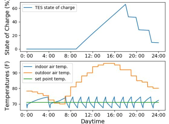
Fig 5 Schedule-based control for TES – (upper) state of charge and (lower) lossless thermal comfort
