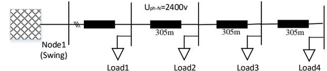
Fig 1 Four-node Test Feeder
