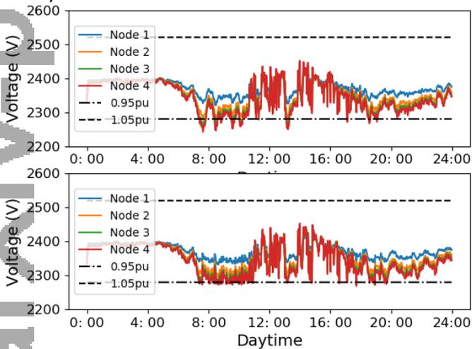
Fig 6 Voltage levels of the four-node system – (upper) before priority-based pass TES control and (lower) after priority-based passive TES control;
