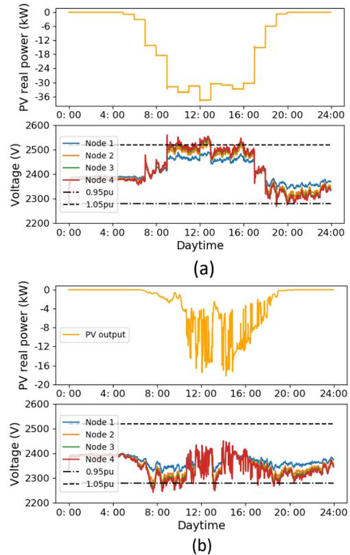
Fig 2 Voltage instability risks under high PV penetration condition: (a) voltage rise during the clear sunny day; (b) voltage sudden drop during cloud passing moments;
