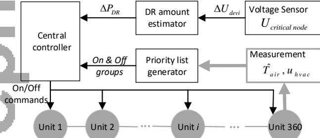
Fig 3 Temperature-priority based control for passive TES
