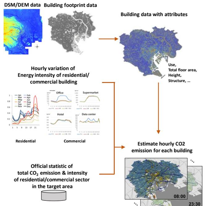
Fig 2 Procedure for estimating the CO<sub>2</sub> emission of buildings
