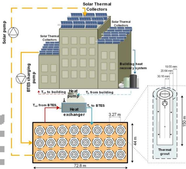
Fig.1. Schematics of the proposed system
