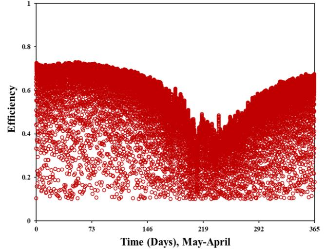
Fig 3. Efficiency of solar thermal collectors for a year
