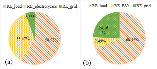
Fig. 1 Self-consumption ratio of zero-energy community with HVs (a) and BVs (b)
