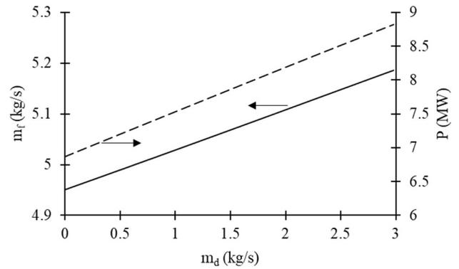
Fig 3 Variations of fuel flow rate ( $m_f$ ) and power output of steam turbine ( $P$ ) with mass flow rate of steam ( $m_d$ ) in steam dryer in the cogeneration system that supplies saturated steam from desuperheater to steam dryer
