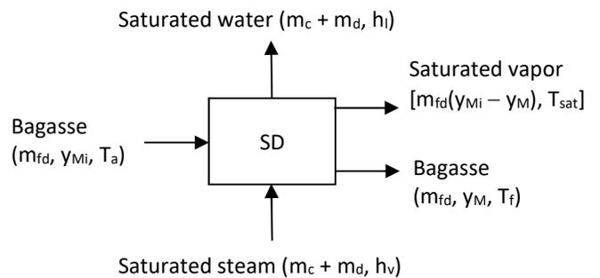
Fig 2 Steam dryer model
