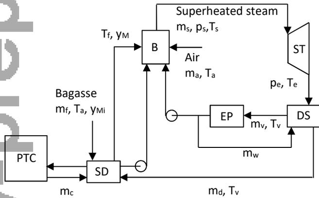
Fig 1 Cogeneration system integrated with parabolic trough collector and steam dryer
