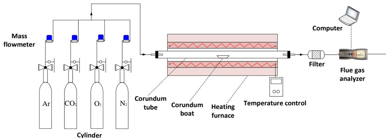
Fig. 1 The experimental system
