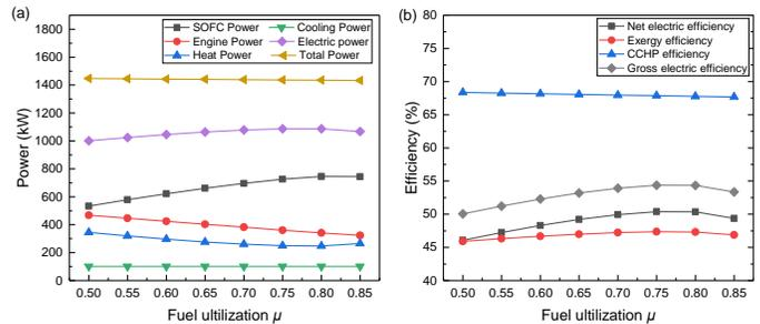
Fig 4 Effects of fuel utilization factor  $\mu$  on system performance
