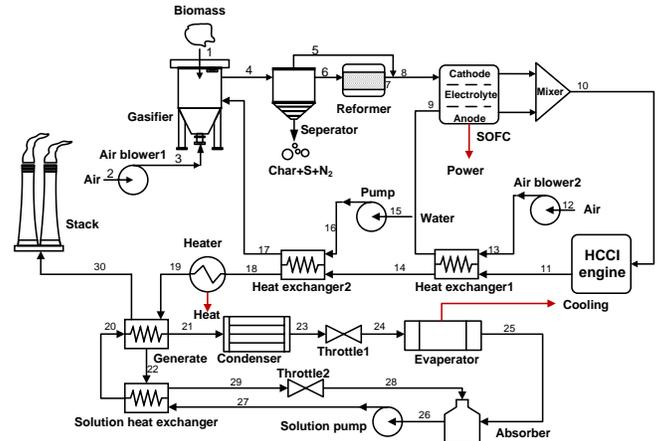
Fig 1 Schematic diagram of CCHP system based on SOFC-Engine and absorption chiller
