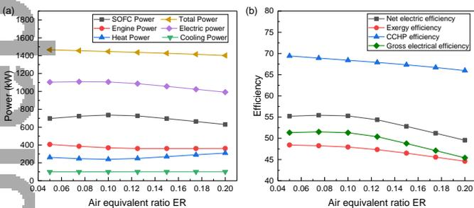
Fig 3 Effects of air equivalent ratio ER on system performance
