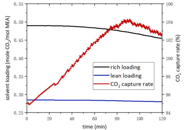
Fig. 6 CO<sub>2</sub> capture rate and solution loading
