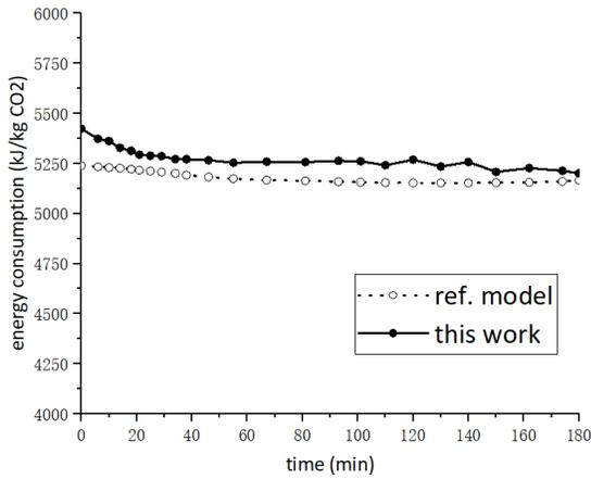
Fig. 4 Validation of stripper: energy consumption
