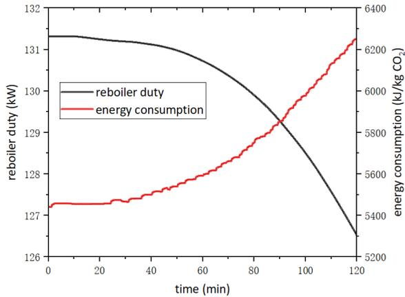
Fig. 7 Energy consumption and reboiler duty
