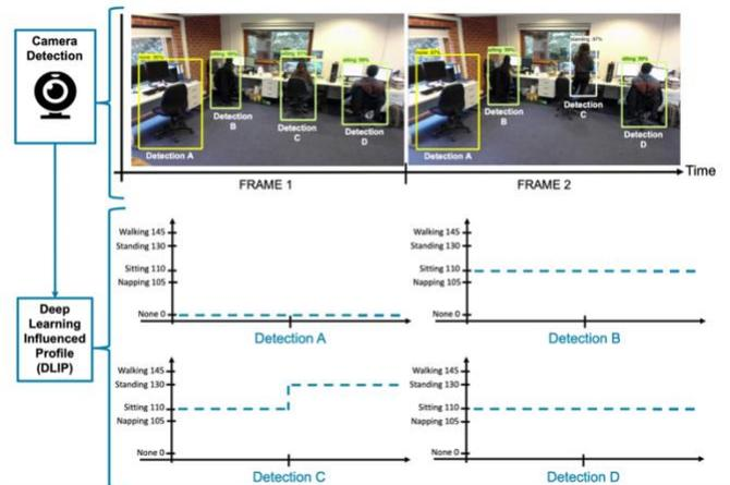
Fig 4 Process of forming the deep learning influenced profile from the application of the deep learning approach for occupancy activity detection and recognition
