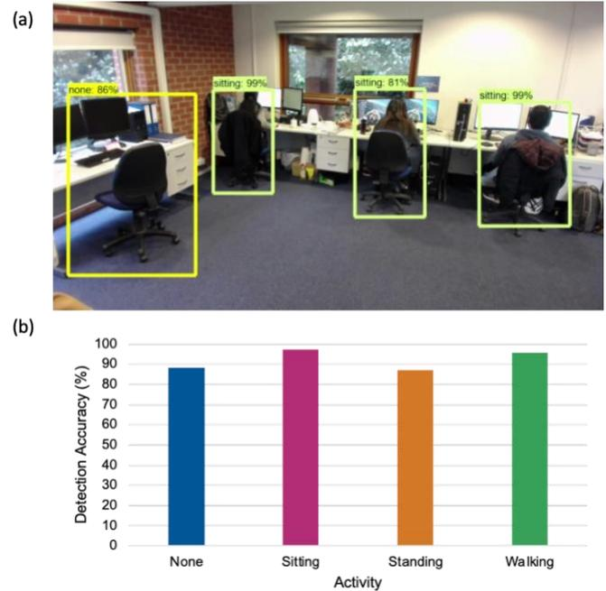
Fig 6 (a). Example detection and recognition result. (b) Detection performance based on each activity
