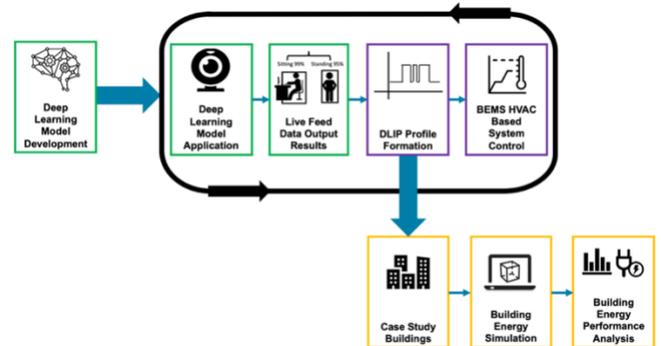
Fig 1 An overview of the proposed framework approach and method
