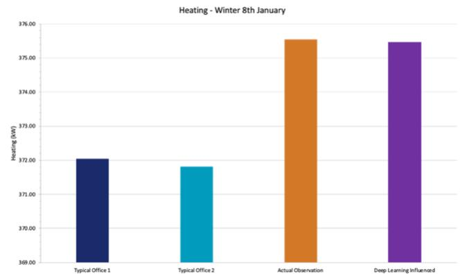
Fig 10 Total heating load for a selected winter’s day based on the assignment of the different forms of occupancy profiles
