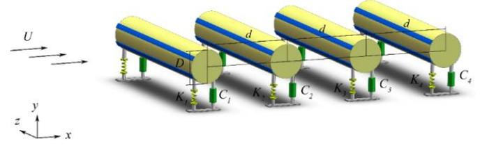
Fig. 1 Schematic diagram of the physical model
