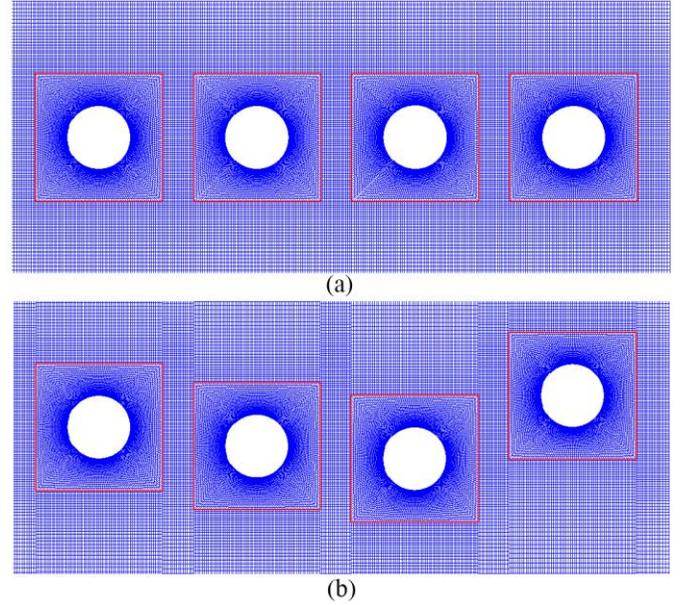
Fig. 3 Close-up of the grid for four cylinders
