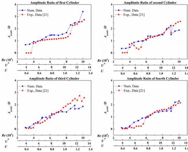
Fig. 4 Amplitude ratios of four cylinders in tandem
