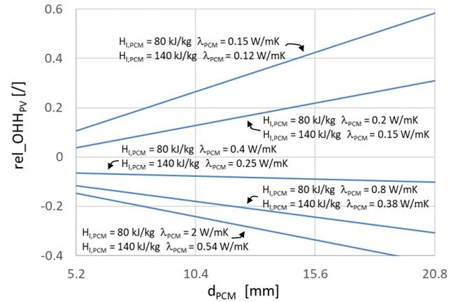
Fig 6 BIPV structure with PCM:  $v_{gap}=1$  m/s,  $d_{glass,s}=4$  mm.
