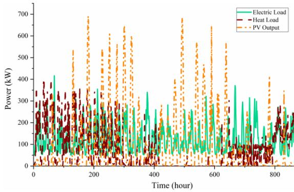
Fig 2 Load curves and PV output curve
