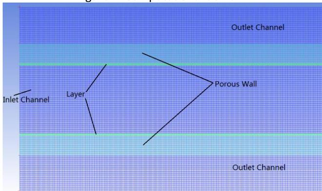
Figure 2. Grid diagram of DPF close to inlet.
